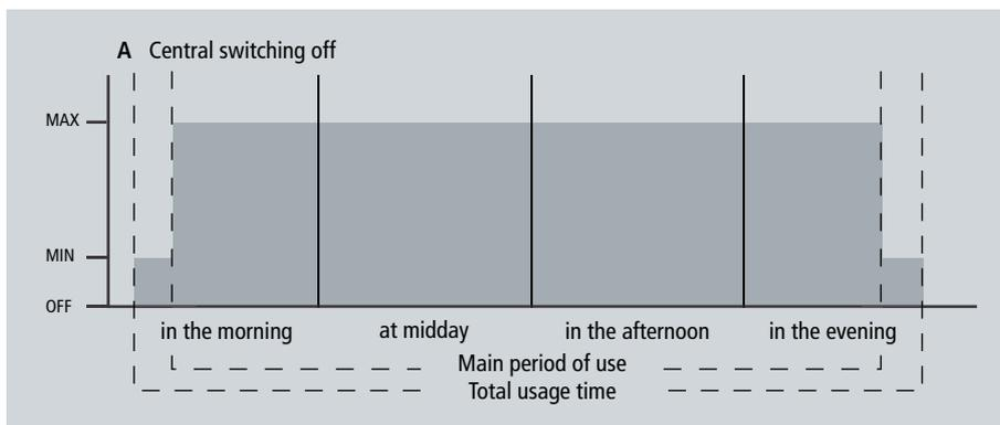
Fig. 2 Saving of energy by central switching off
