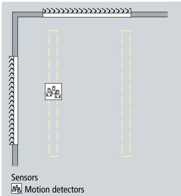
Fig. 7 Use of a motion detector in the combination of presence-dependent and daylight-dependent lighting
