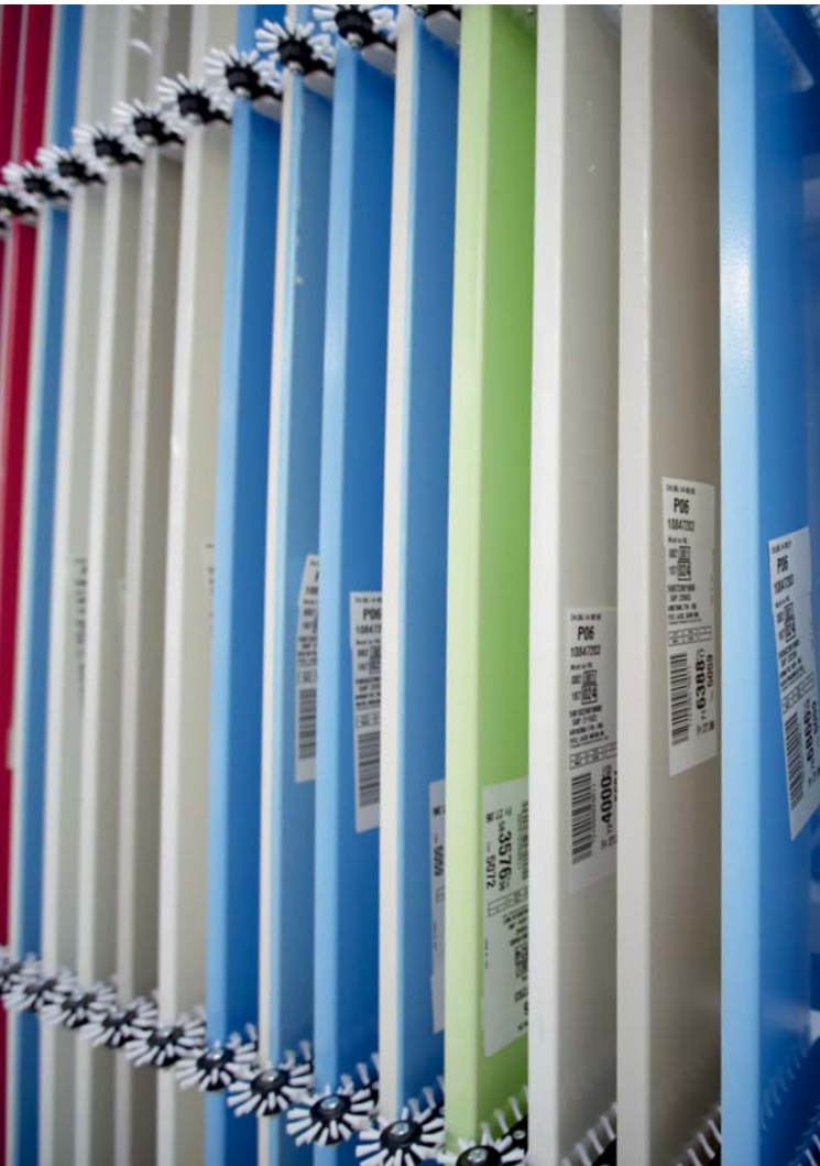
Each element can be very clearly assigned to the correct kitchen furniture via unique barcodes.
