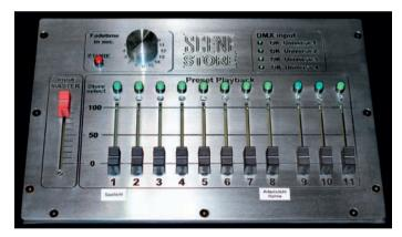
Scenestore is a secondary lighting control system developed by Stage Entertainment. The system is independent of the main lighting control console and used for rehearsals as well as for backup in the event of a fault.
