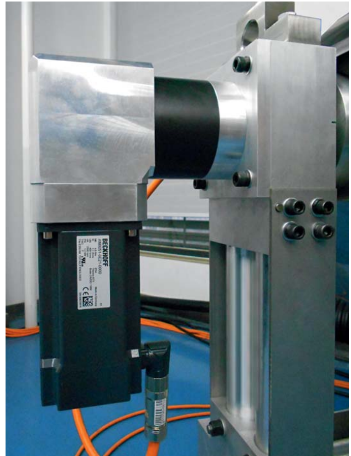
When connecting the AM8000 servomotors, only one cable needs to be laid, since the One Cable Technology (OCT) combines power and feedback systems.
