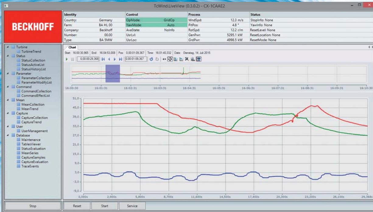
Fig. 4: The visualization is used to display current states, values, and settings.
