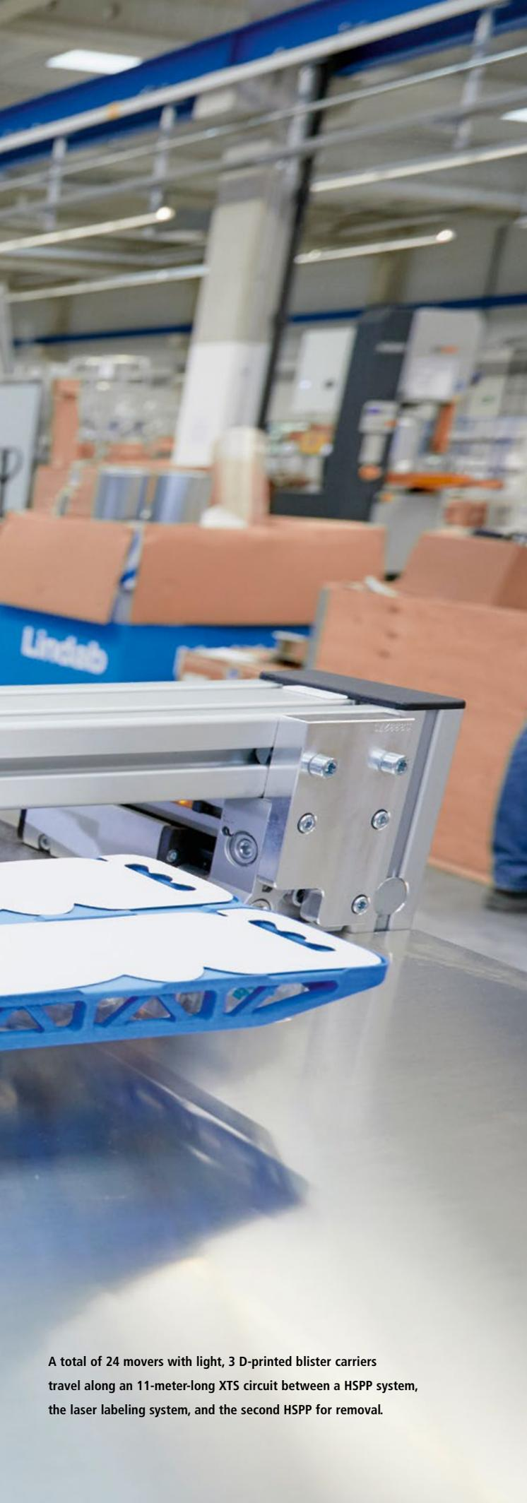
A total of 24 movers with light, 3 D-printed blister carriers travel along an 11-meter-long XTS circuit between a HSPP system, the laser labeling system, and the second HSPP for removal.
