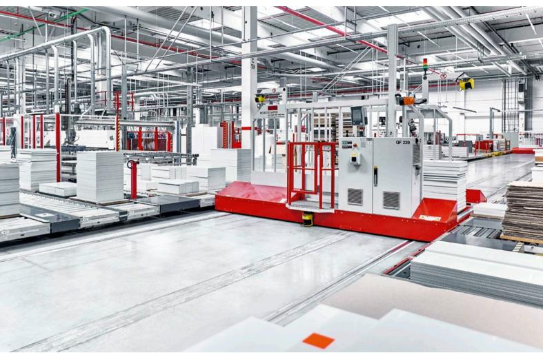
The different traverse conveyor vehicles can travel at speeds of up to 85 meters per minute without endangering worker or forklift through traffic.
