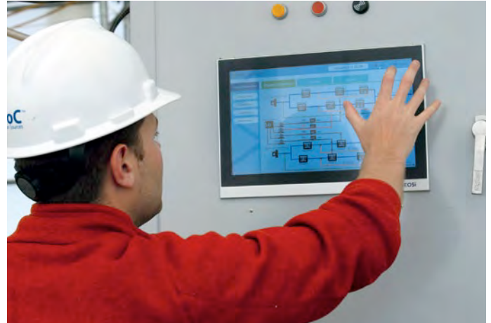
The CP2216 multi-touch Panel PC from Beckhoff runs the HMI software from EOSi and the TwinCAT PLC software.
