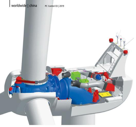
Predictive maintenance with TwinCAT Wind Framework software uses ultra-fast EtherCAT communication to monitor the main components in a wind turbine nacelle (in this case with direct drive), such as rotor blades, hub, pitch system, generator rotor, generator stator, gear system, wind measurement system along with the foundation plate and tower frame.
