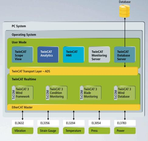
The TwinCAT-based CMS acquires and analyzes vibration data from the online generator bearing and saves it at high speed in a local database via TwinCAT Wind Framework.
