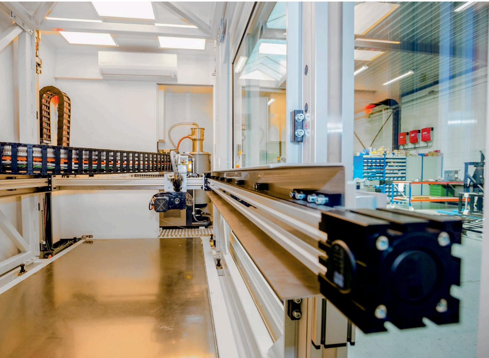
XYZ portal as the 3D printer's drive: Toothed belts drive the X and Y-axes; an additional computing procedure converts the desired X and Y coordinates for correct toothed belt drive control.
