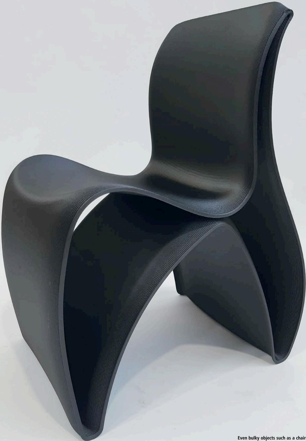
Even bulky objects such as a chair can be manufactured rapidly with Colossus, one of the largest transportable 3D printers in the world.
