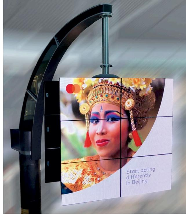
The LED screens can be dynamically combined and separated again to form a wide range of shapes with two, three, four and six displays.
