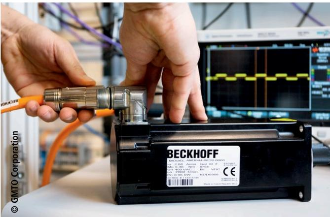
Beckhoff AM8000 servomotors are specified throughout the telescope design, which includes more than 3,000 axes of motion.
