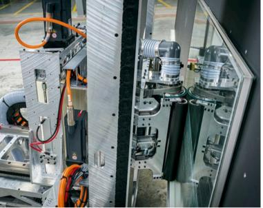
Above: AX5000 series Servo Drives from Beckhoff power all axes of motion with space-saving One Cable Technology that provides power and position feedback in a single cable.
