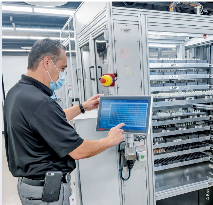
Beckhoff multi-touch Control Panels are used for greater visualization of milling processes.
