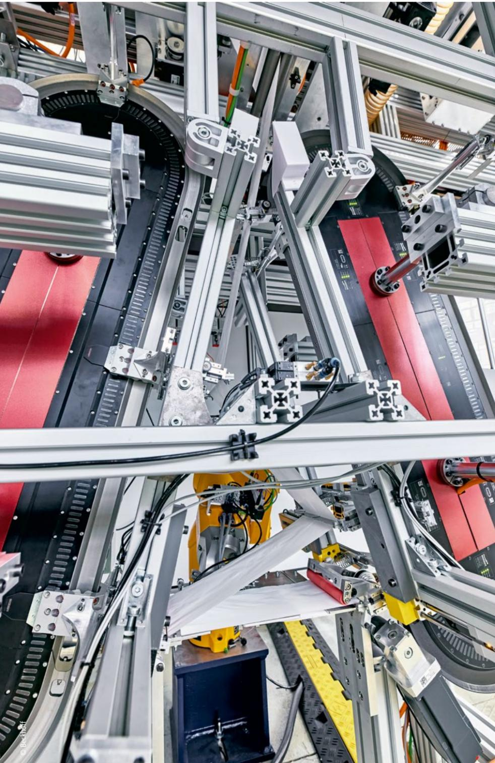
For continuous Z-folding, the cut electrodes must be fixed on the separator film. With two XTS and their rotating grippers, the cells can then be folded quickly and precisely.
