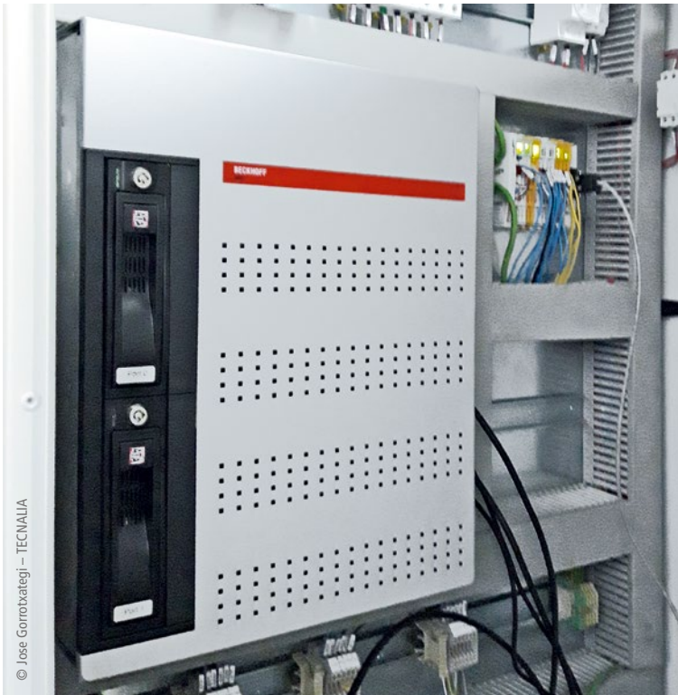
A C6650 control cabinet Industrial PC takes over the central control of all axes and the positioning of the cable robot using various nautical sensors.
