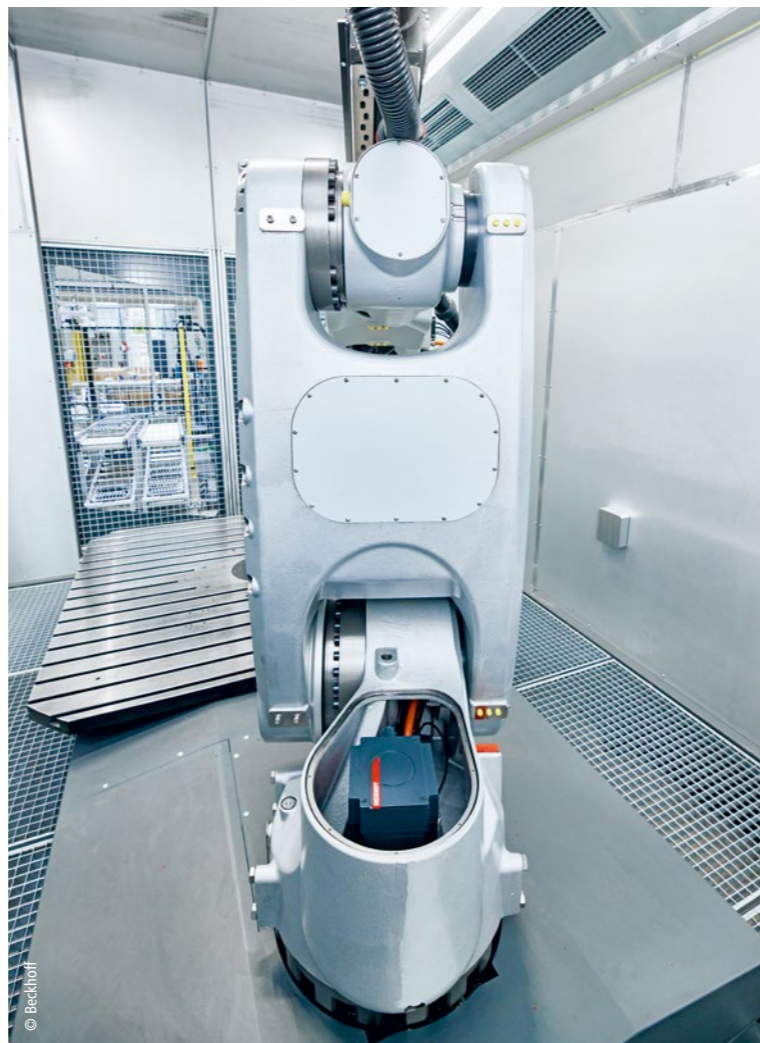
In the robot, Beckhoff AM8000 servomotors together with the encoders on the drive and output sides ensure precise movements.
