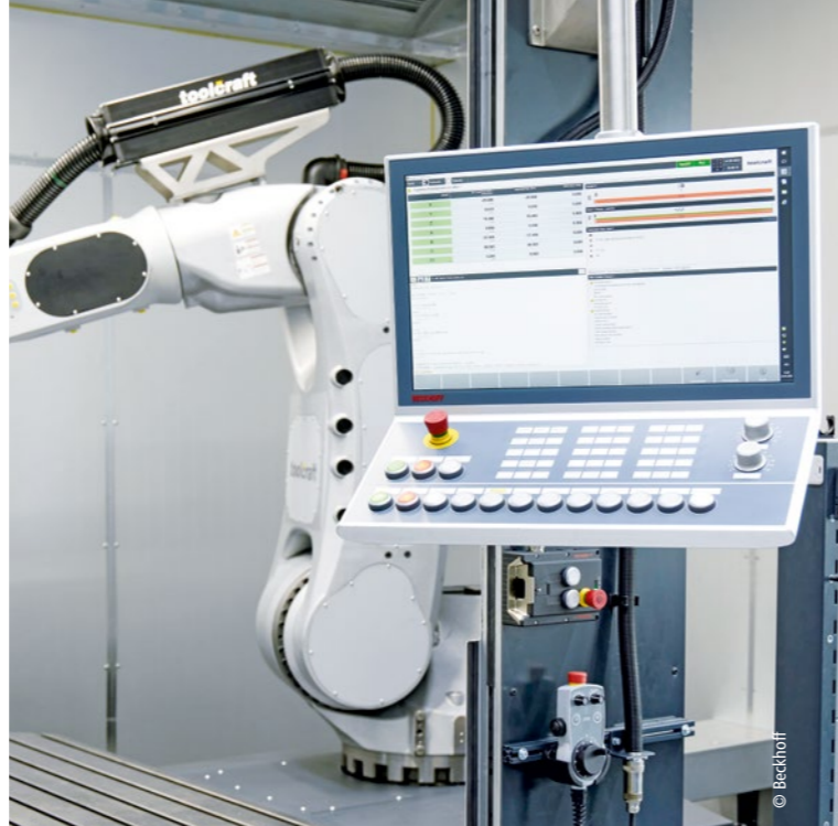
Operation and path planning are carried out in G-code, just as the 5-axis CNC, and visualized on a customer-specific CP3921 multi-touch Control Panel.
