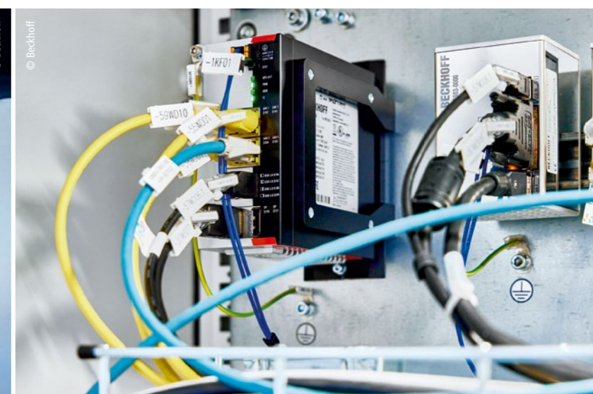
The powerful C6030 ultra-compact Industrial PC controls all machine and operating processes.
