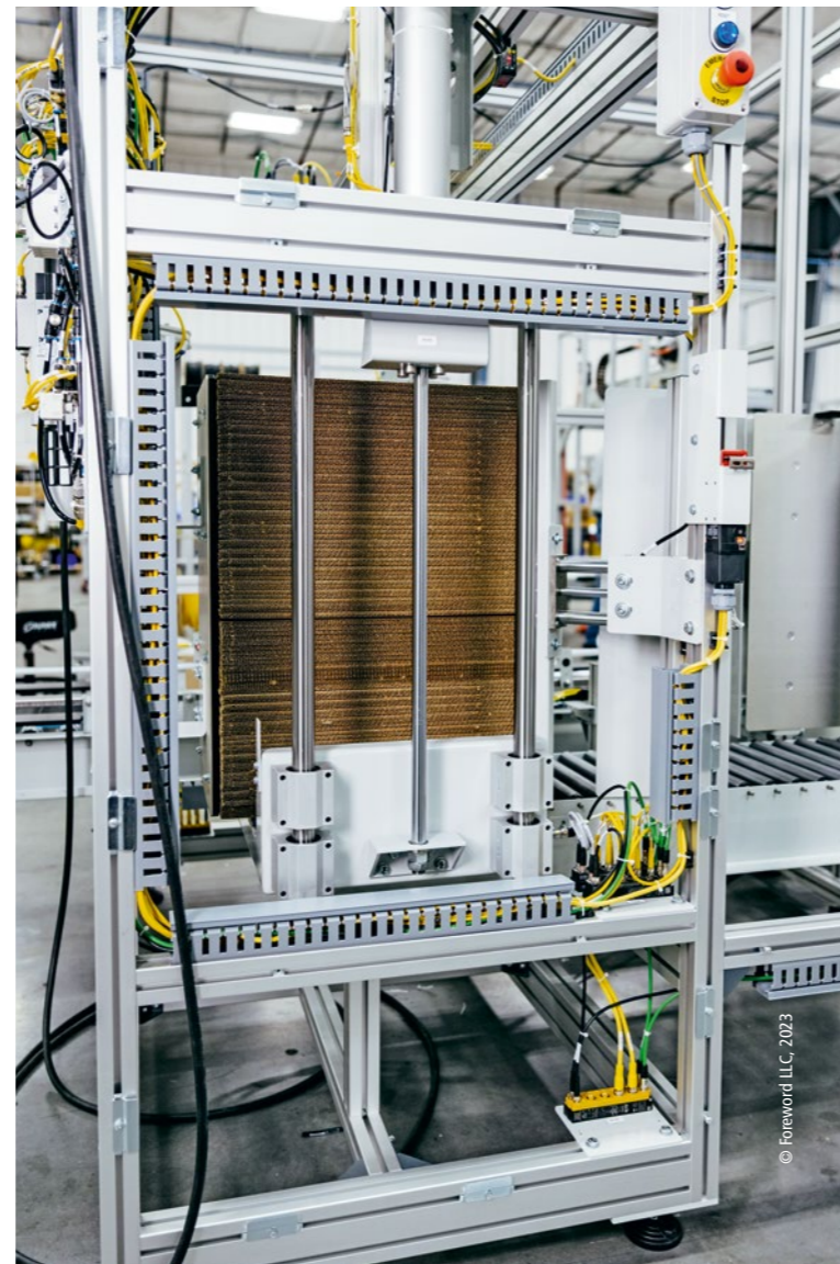
The case erector folds the bottom of the corrugated boxes while the bagged medical products are being prepared.
