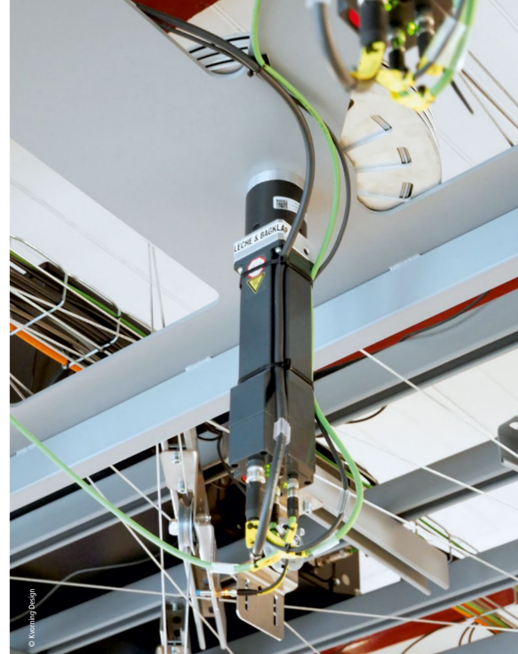
AMI8100 distributed servo drives complete with backlash-free permanent magnet holding brake and TwinSAFE STO/SS1 safety function move the smaller body parts, with everything controlled via TwinCAT alongside the AM8000 synchronous servomotors.
