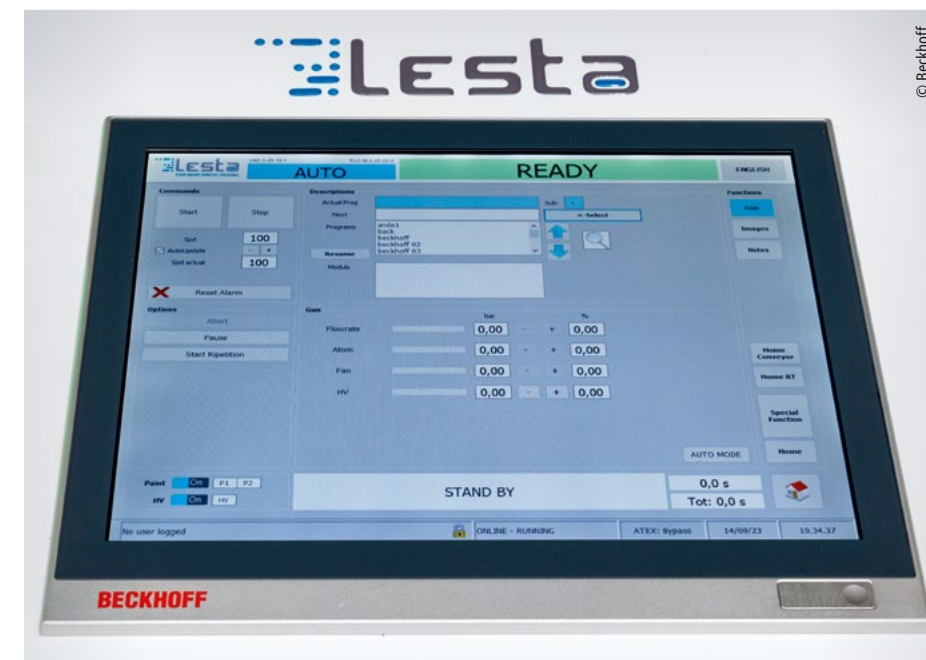
Lesta uses a CP2915 multi-touch built-in Control Panel to operate the painting systems.
