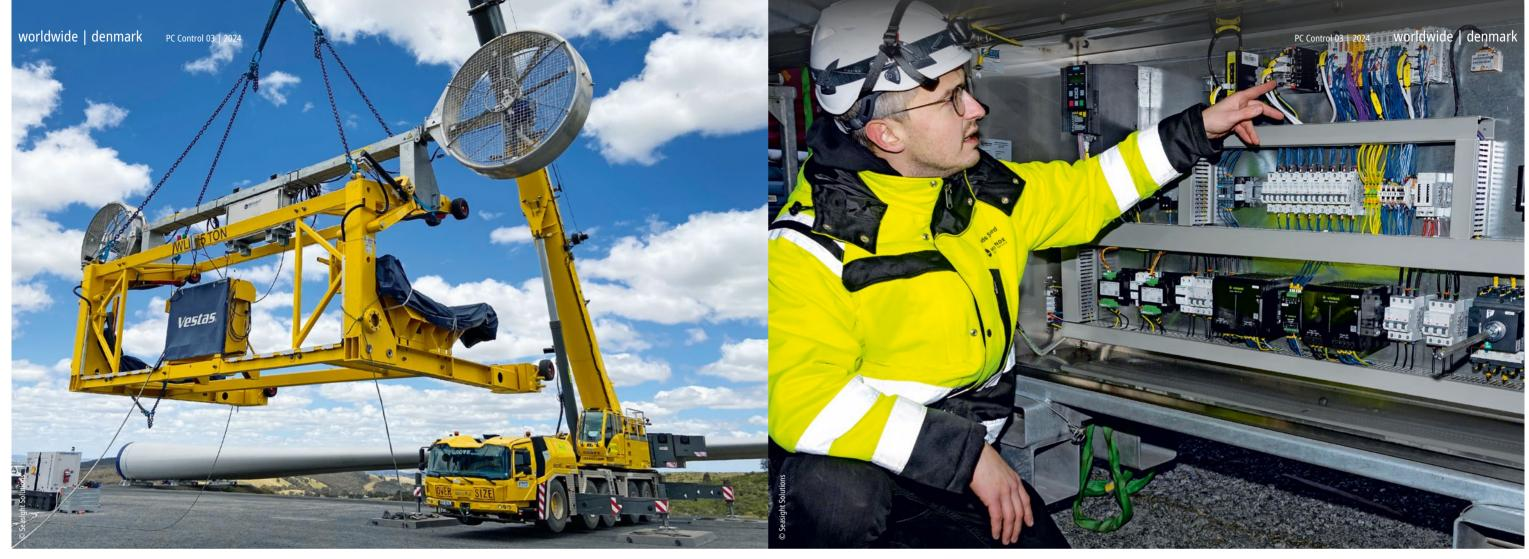
A high-performance automation platform is needed to keep the positions of the rotor blades precisely in place – even in strong winds. Seasights Solutions have found the ideal control solution for this in the form of PC-based control and TwinCAT.
