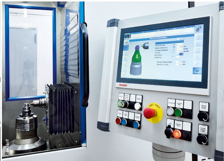
The tools and jobs are selected via a CP2916 multi-touch Control Panel, which is connected to the CX5140 Embedded PC in the control cabinet.
