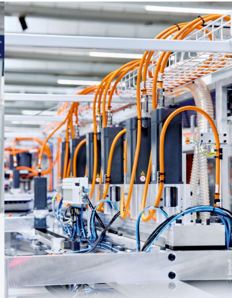
Numerous AM8000 servomotors ensure highly dynamic and precise process sequences.
