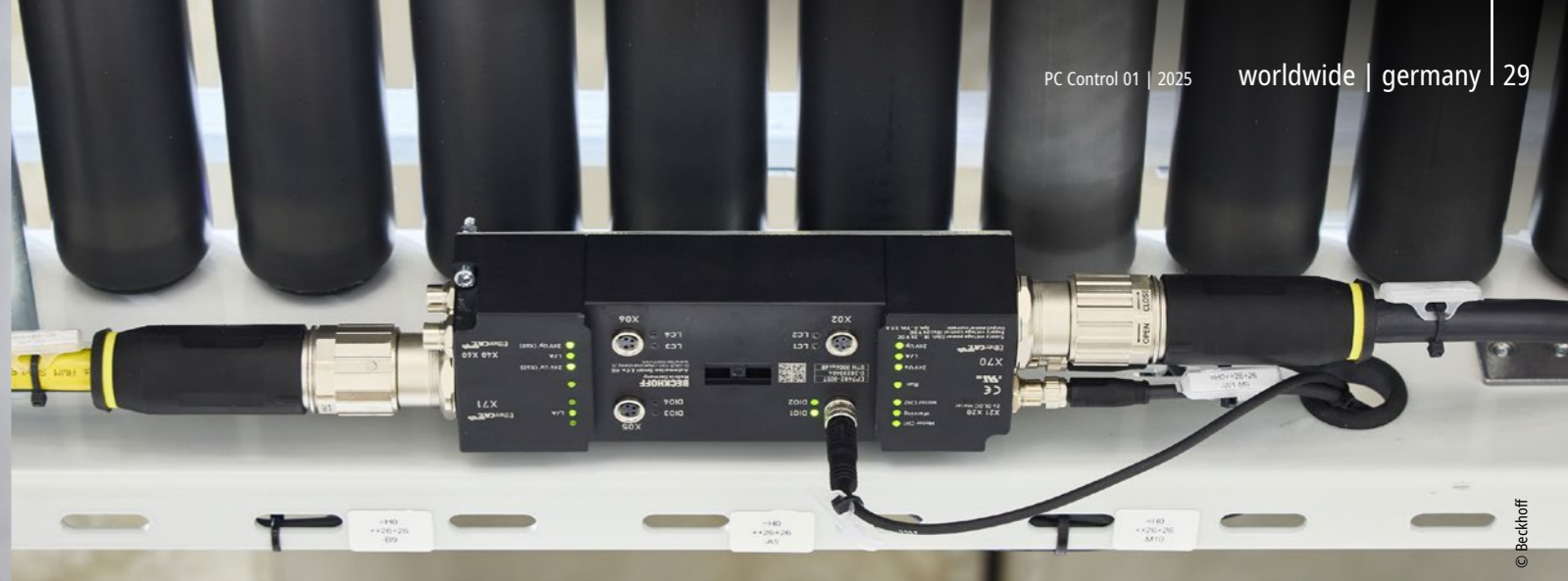
Special components such as barcode scanners are integrated via the integrated EtherCAT junction of the MDR controller.
