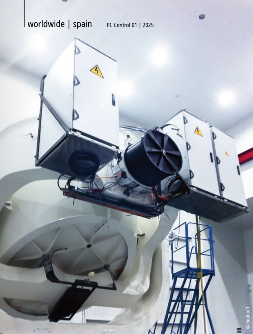
The QUIJOTE I telescope with the axes for vertical alignment (elevation) and instrument cabinets.
