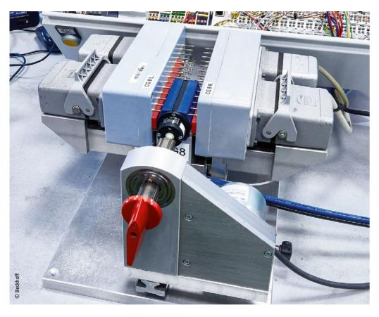
Left: Reducing the EtherCAT cycle to 20 µs enables rapid transmission of the 830,000 input and output values recorded during the test.
