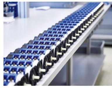
Every cam switch at Kraus & Naimer undergoes thorough testing of its switching patterns and functionality on a range of test benches.
