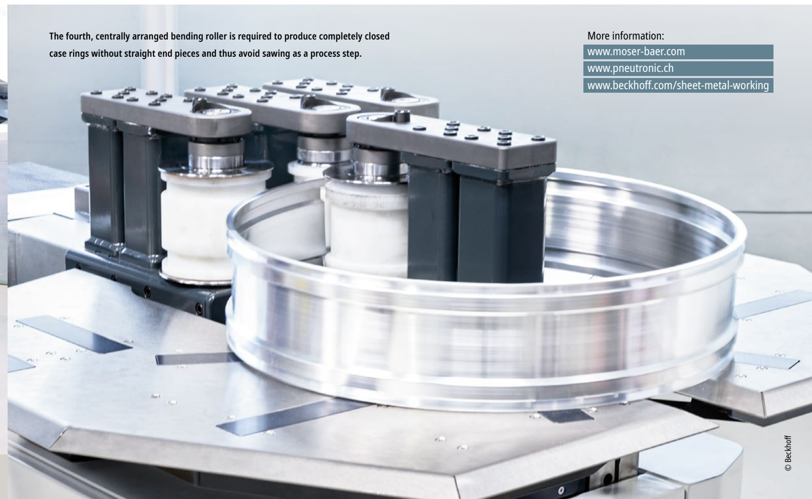
Without the space-saving AM8000 servomotors and One Cable Technology as the connection technology, it would not have been possible to design such a compact roller bending machine.
