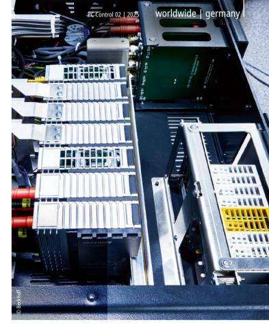
In addition to the EJ modules (right) and EtherCAT Terminals from the EL series, the MTS also uses the high-precision EtherCAT measurement terminals from the ELM series (left); shown here in the MDU module.
