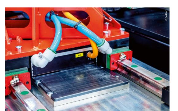
Highly dynamic AL8000 linear motors move the gantry axes of the laser processing center with speed and precision.
