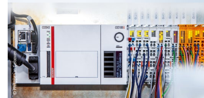
CNC Solutions has been using PC-based control and CX2043 Embedded PCs to control a wide variety of projects for the last two years.
