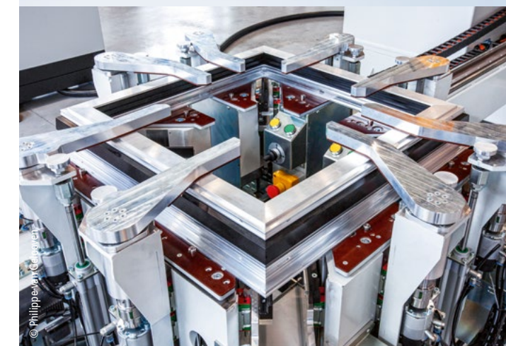
Prior to pressing the frames, the fixings are positioned according to the window size.
