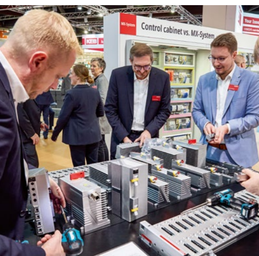
The decentralized MX-System is the first to achieve completely control cabinet-free automation of machines and systems with PC-based control.
