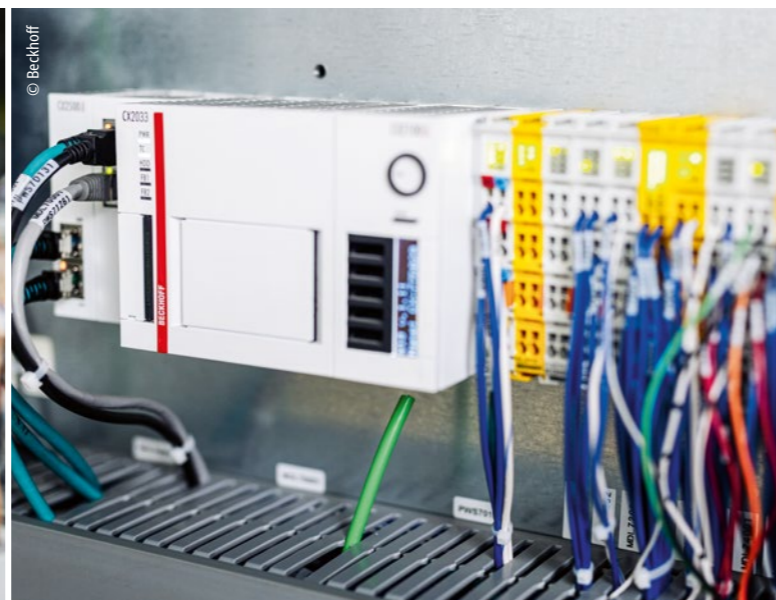
The Beckhoff CX2033 Embedded PC functions as the sole machine controller for the 1400-GEC mailer packaging machine and contributes to boosting scan times.
