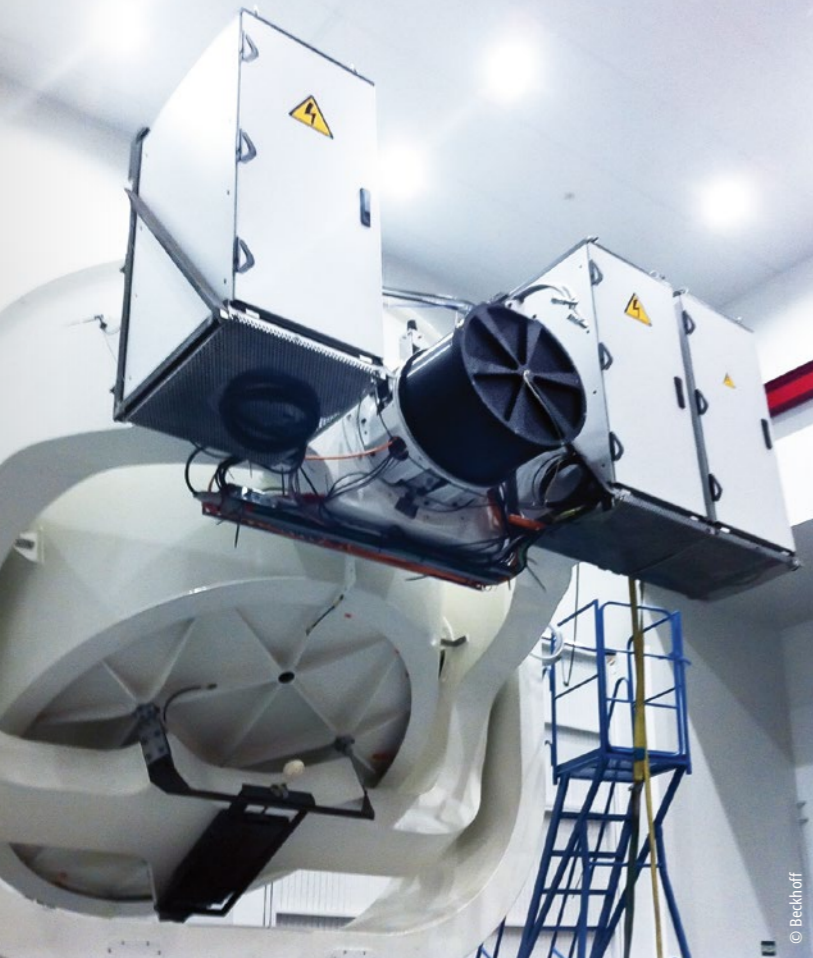
The QUIJOTE I telescope with the axes for vertical alignment (elevation) and instrument cabinets.
