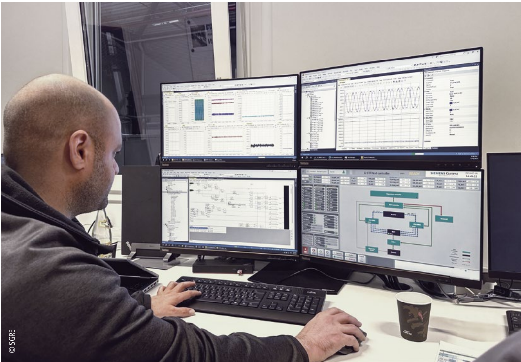
Beckhoff TwinCAT software plays an important role in the SGRE test rig, including TwinCAT 3 Scope View for data analysis (both top screens), TwinCAT 3 Target for Embedded Coder® (bottom left), and TwinCAT 3 HMI for convenient system operation (bottom right).
