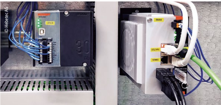
TwinCAT and C6030 ultra-compact Industrial PCs are used to control the many presses for precise leveling, uniform feed, and exact alignment of the tunnel elements.
