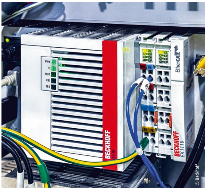
The CX5140 Embedded PC forms the powerful control core of the injection molding machines.
