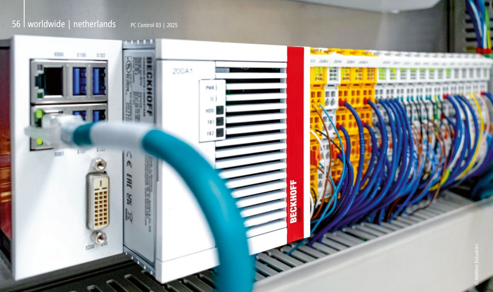
Additive Industries and Cordis rely on a CX5230 Embedded PC with TwinCAT for the control technology.
