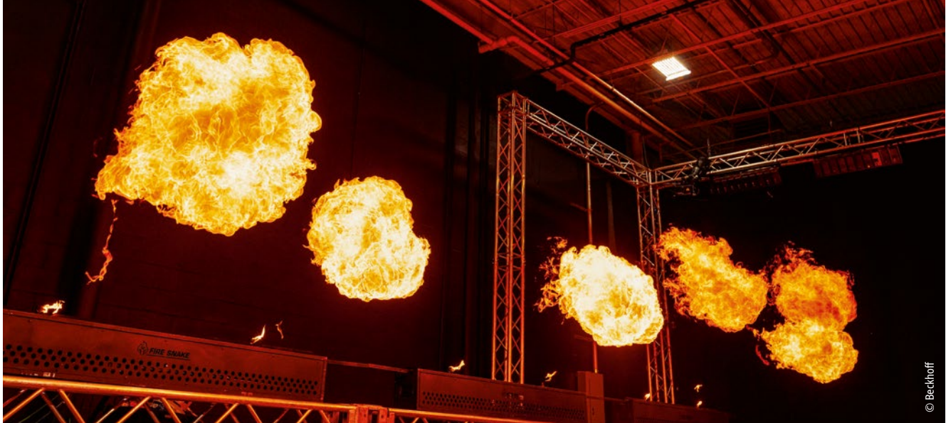
The propane-powered burners generate continuous flames with an adjustable height of up to 1.80 m, as well as rolling fireballs using bursting valves.
