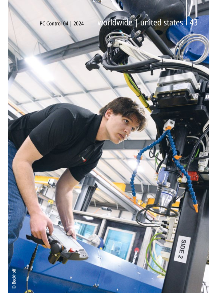
Using Hot Connect capabilities in EtherCAT, the Robotic Twin system can quickly change end-of-arm tooling to switch inspection types, increasing flexibility.
