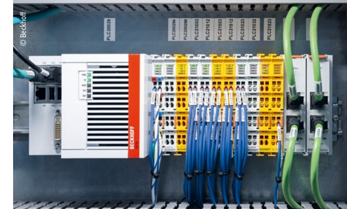
A CX5130 Embedded PC from Beckhoff serves as the central machine controller for the robotic testing center.
