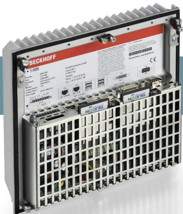
Flying by Foy’s control solution is mounted in a 3.5” rack using a Beckhoff C6515 Industrial PC.
