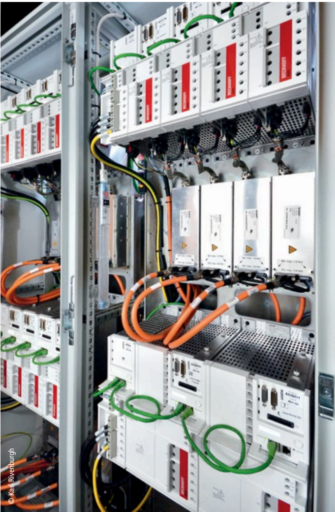
Action and spectacular effects are the heart of any performance: for motion control, Hudson Scenic leverages AX5000 series EtherCAT servo drives and AM8000 series synchronous servomotors with OCT.
