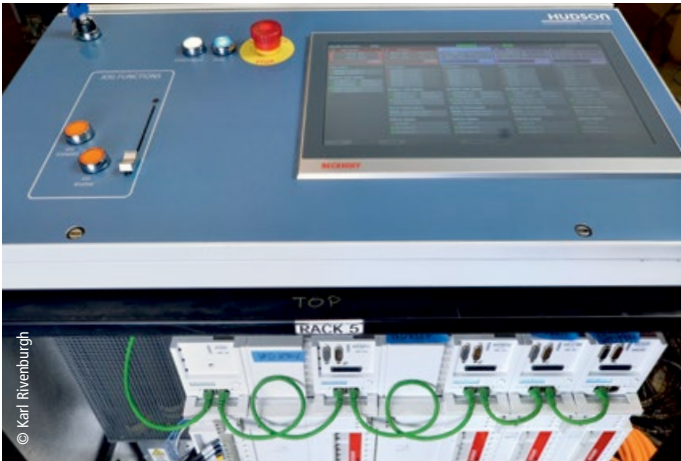
Displaying the HMI programmed by Hudson is a series of 15-inch Beckhoff CP2916 multi-touch Control Panels.
