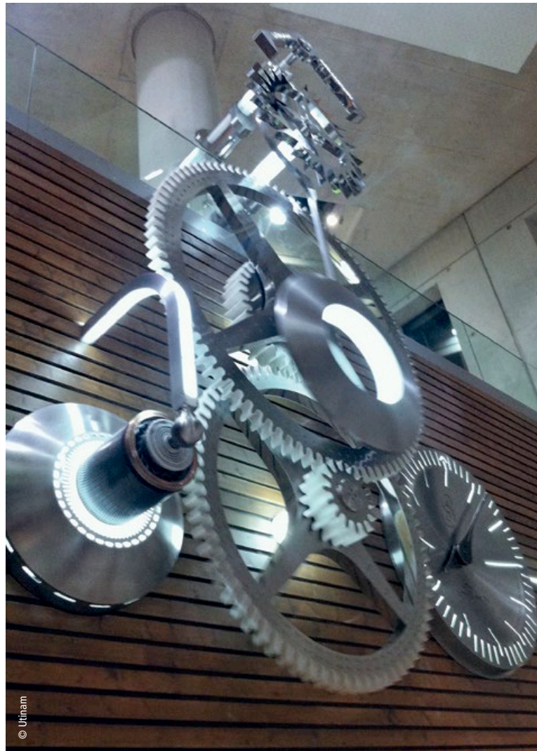
The eye-catching clock which Utinam designed for the TGV station in Besançon has no housing, making its mechanisms fully visible. With its considerable height of six meters, it stretches over two floors. The escape wheel, which links the mechanisms to the pendulum, has a diameter of 1.44 meters while the hour wheel measures 2.85 meters.
