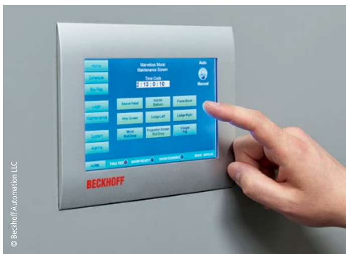
A CP6706 Panel PC running TwinCAT 3 software automates the entire Northwoods Friends Show.
