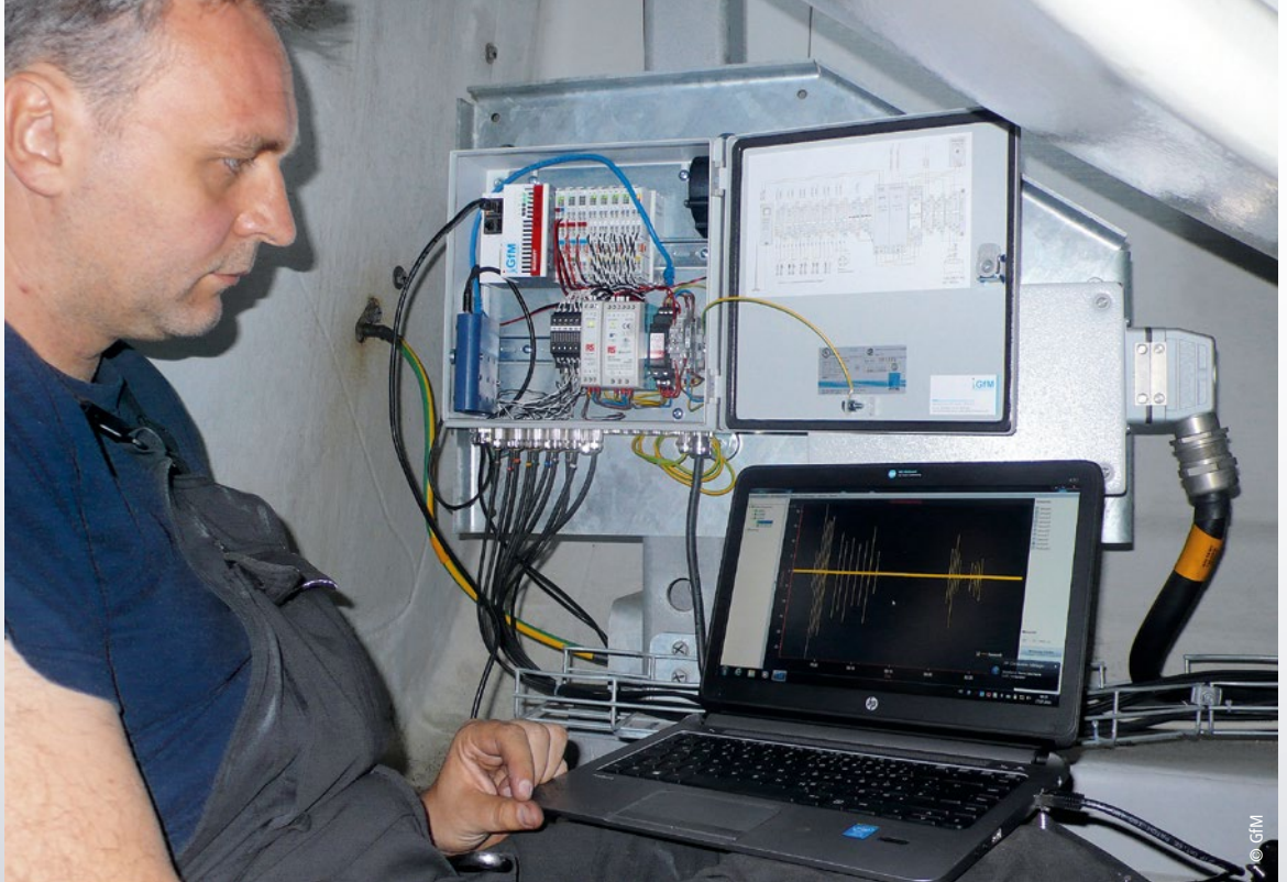
GfM staff engaged in testing acceleration sensors connected to the Peakalyzer.
